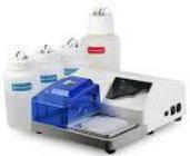
The DIAAMW-3000 automatic plate washer is used to clean some residual substances after the detection of ELISA plates, so as to reduce the errors caused by the residues in the subsequent detection process. It is widely used in scientific research laboratories, quality inspection bureaus, agricultural animal husbandry, feed enterprises, food enterprises and other testing fields.
